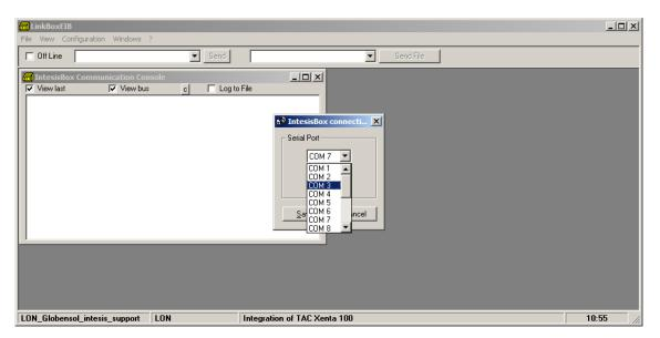
3. Click the checkbox next to *Offline* word below LinkBox Menu. It should change to Online, and some output must appear at *IntesisBox Communication Console* window.
