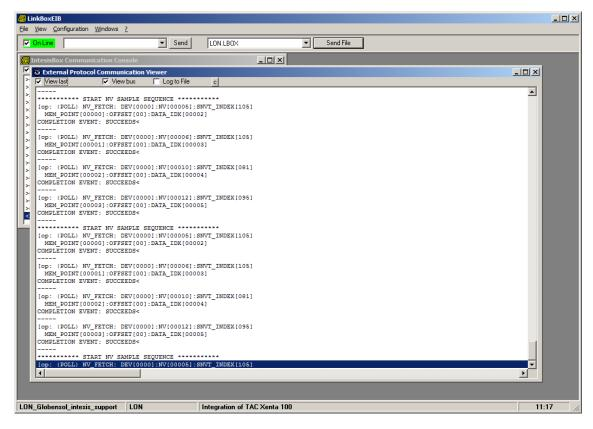
These pose as the query commands the IntesisBox is triggering to the LonWorks device being integrated.
