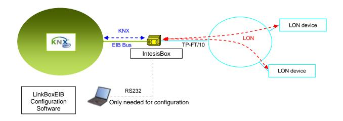
Integration of LON and KNX using IntesisBox KNX - LON gateway
